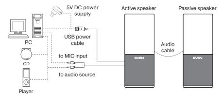
Fig. 2. Connection diagram
