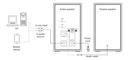
Fig. 2. Connection diagram
