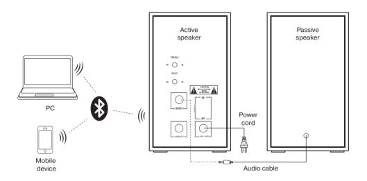
Fig. 3. Connection diagram audio source via Bluetooth-module
