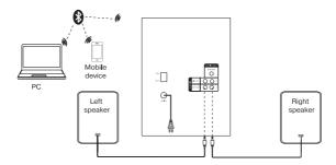
Fig. 6. Bluetooth module connection diagram
