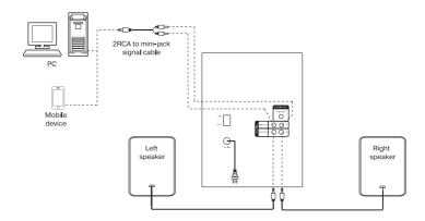
Fig. 5. Connection diagram
