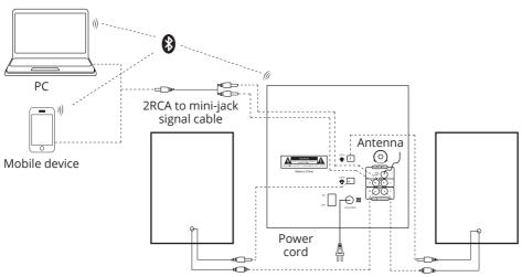
Fig. 5. Audio sources connection diagram
